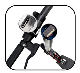
Gently introduce the handlebar assembly into the handlebar stem, and push home.
