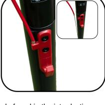
Attention: Take control of the handlebar stem as it collapses to the folded position.
