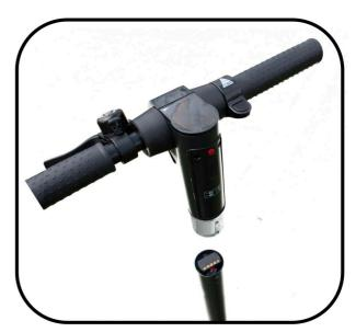
Align the two bolt holes of the handlebar assembly neck with the holes in the stem. Re-position the Locking Hook and secure the two bolts through the three parts using the Allen key provided.
