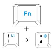
Press Fn + any number from 1 to 8 to switch between LED modes.
